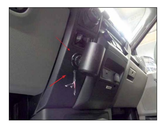
Secure pod with two screws in the location shown.
